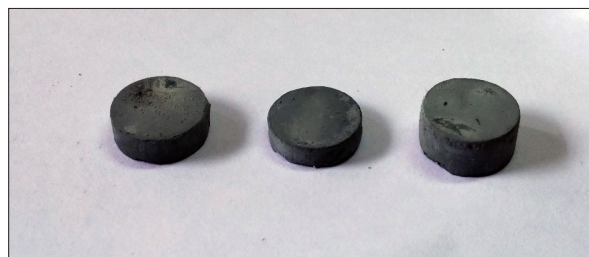
Fig.2. compacted pure silicon after pressing
